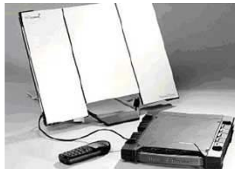
The BGAN Explorer 700 Satellite Communication System.
